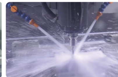
Side Surface Drilling
