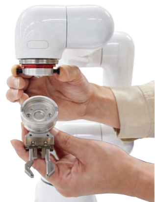
Push in the pusher to attach/detach a tool.
